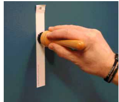
Figure 3. Adhering Product strips
