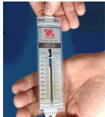
Figure 4. Zeroing the scale
