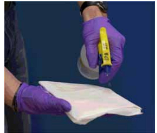
Figure 6. Soaking a lint free cloth
